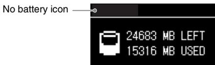
To recover, fully charge the battery using the supplied AC power adapter. Do not remove the adapter while charging is in progress.
