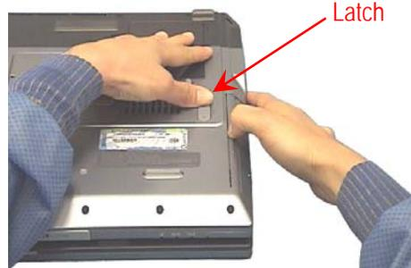
**Step 5.** Unlock the ODD Latch.
